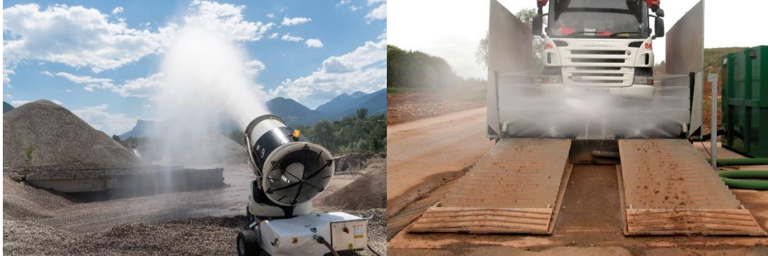
Figure 5.1 Dust suppression cannon (left) picture source: https://www.tecpro.com.au/product/v22-dust-controller/ and wheel wash facility (right) – picture source ( https://www.agg-net.com/resources/articles/loading-hauling/wheel-washers )
