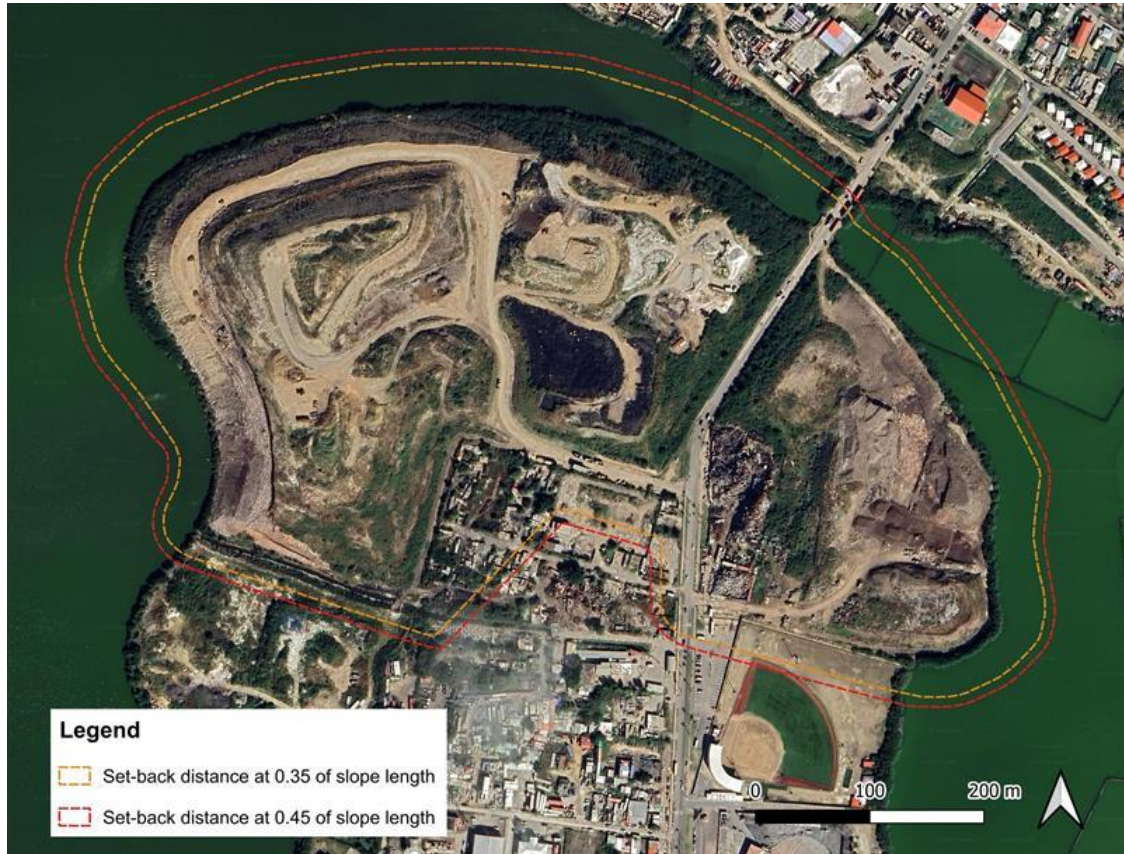
Figure 2.2 Set-Back Distance at 0.35 and 0.45 times slope length
