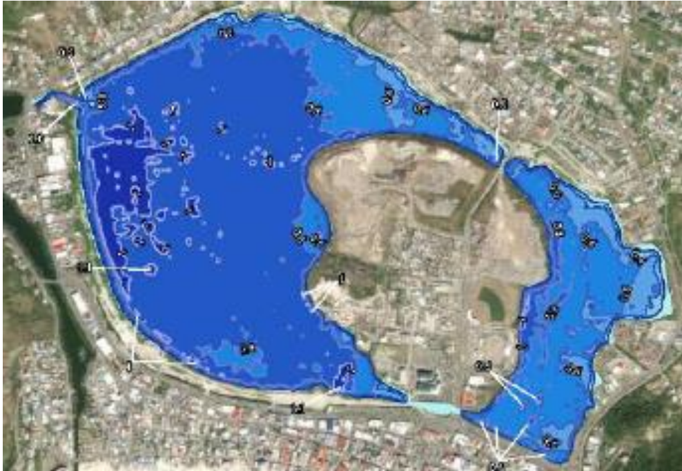
Figure 3.9 Bathymetric Readings for the Great Salt Pond (University of South Florida Water Institute)
