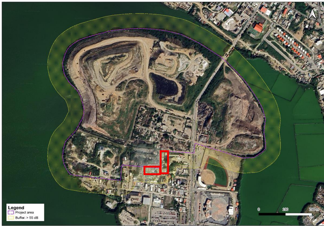
Figure 5.2 Map with the maximum extent where noise levels are exceeding 55 dB(A) assuming all activities are a single point source. Area in red is closest houses
