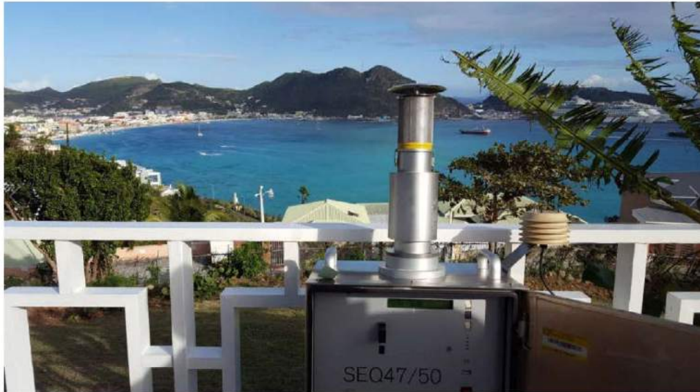
Figure 7 Leckel 24/7 dust sampler at Belair (location C)
