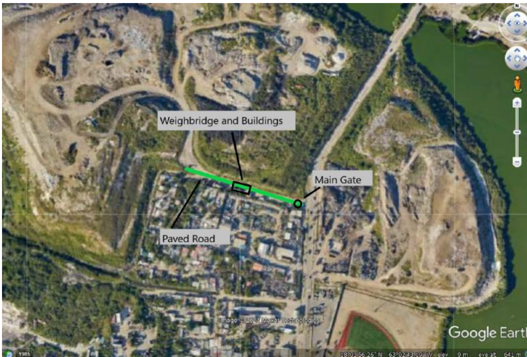
Figure 1.9 show details of the location of works related to the paving of the existing access road (Brine Drive) to the MSW landfill, the placement of a main gate, weighbridge scale and buildings.
