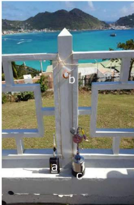
Figure 10 Pump (a) with charcoal tube, 3M™-badge (b) for passive sampling and metal canister with restrictor (c) for a sampling time of \pm 2 hours at Belair (location C).
