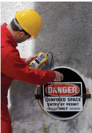
Confined space testing with the MultiRAE Lite
