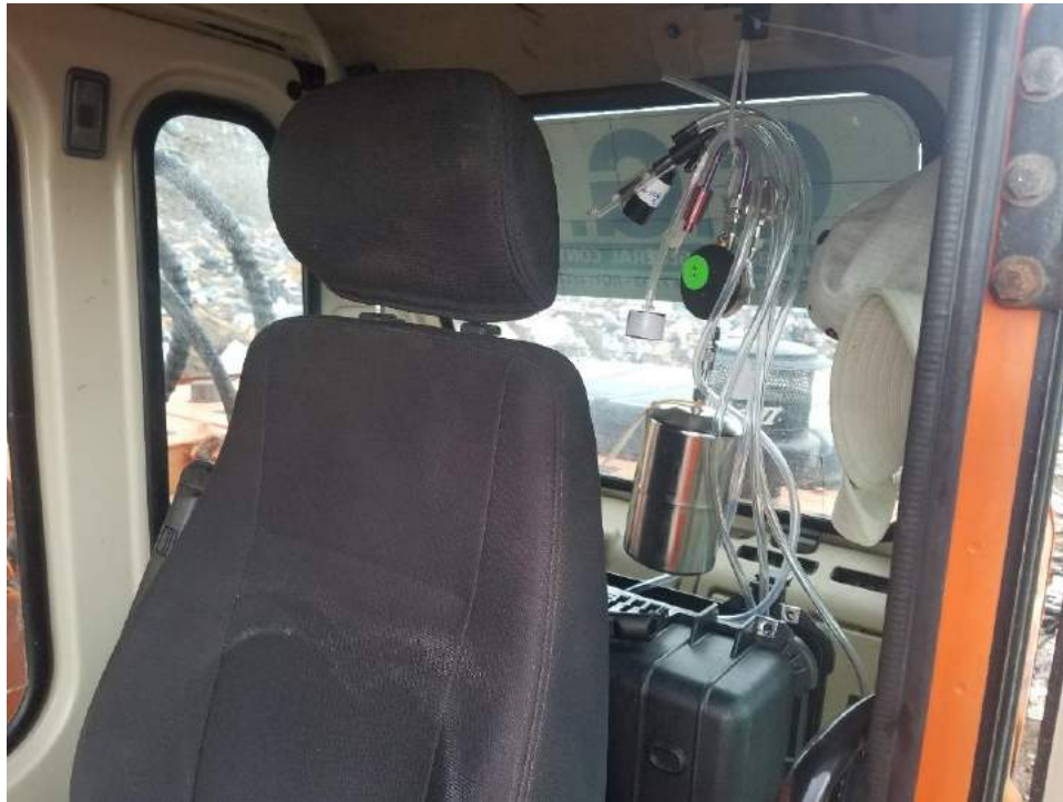
Photo 3 – Typical Personnel Sample Placement
