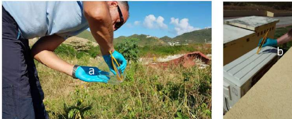
Figure 12 Dust sampling: wiping a Petri dish (a) and a 'historical wipe' (b).
