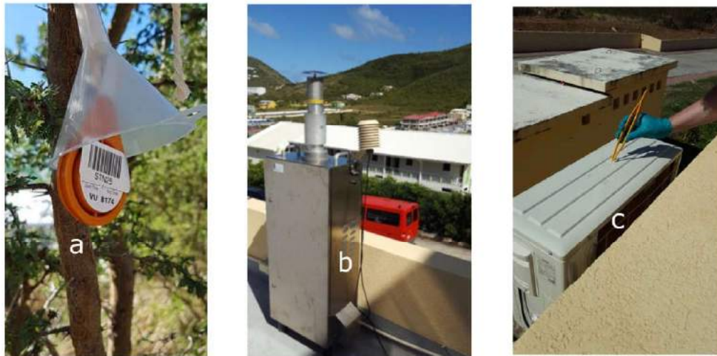
Figure 1. 3M badge for passive sampling at location 1 (a), Leckel filter equipment at location D (b) and swiping dust for historical interpretation (c).
