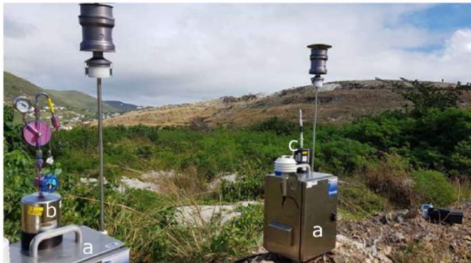
Figure 2. Two KFG dust samplers (a), canister (b) and pump with sorbent tube (c) at VROMI yard (location 4).
