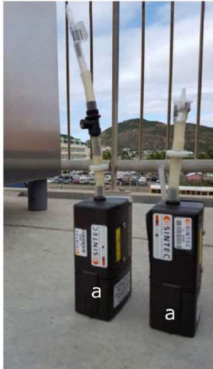
Figure 11 Pumps with active carbon tube (a) and aldehyde cartridge (b)
