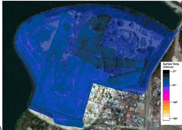
Figure 3.6 June 2018 Aerial Infrared Thermal Survey of MSW Site
