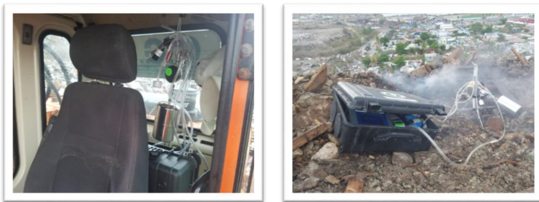
Figure 2. Pictures indicating the locations of the monitoring equipment (left: in the cabs of vehicular equipment driven by operators, and right: in the smoke plumes)
